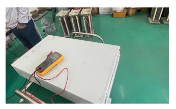
Customer use list and step function to simulate parts of operation condition. Test result meets the requirement; voltage rise time <15ms(no load), <85ms(full load), completely satisfy the requirement of LVRT of PCS. Adjustable output voltage from 0-1000V cover customer's requirement in voltage. Customer speaks highly of the product.
